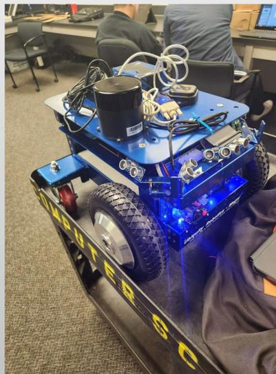
Ubiquity Rover and Rover with Lidar Bar Attached
