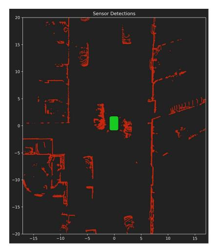
A Python program named generateLidarPlo.py was implemented to create the plots, leveraging the matplotlib library. The program would take the lidar detections data from the given dataset and mark a small red dot on the plot for each detection. The format of the plot was built with the following code snippet:
