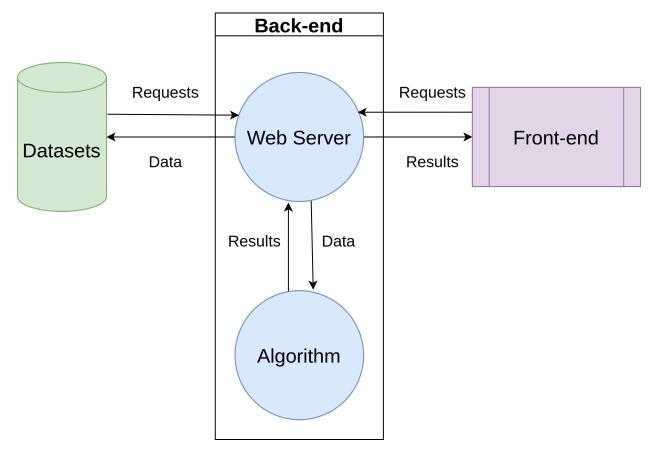
The picture above is a general overview of the whole project. The project consists of a total of three major components, namely the front-end, back-end, and algorithms.
