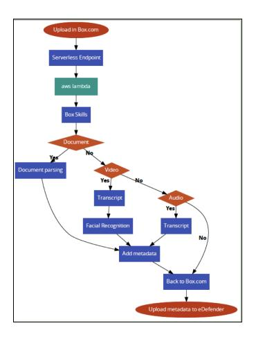
The data flow in our project is as shown in the figure above, starting with a user uploaded video to an enabled Box.com folder (enabled with a Box Skill). Once the video or document is fully uploaded to Box.com, the site will check its extension type to confirm if the call needs to be triggered and then triggers an event to AWS along with the data of the video.
